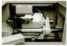
3.7kW oil coolant built-in motor is adopted on Main spindle, and C-axis function is carried on Back main spindle. (Simple belt C-axis)
